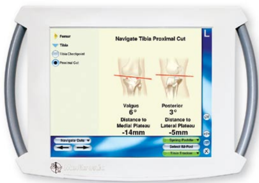
This CAS screen provides real time information about the exact position of the bones and allows for precise cuts for placing the prosthesis.
