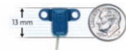
Miniaturized AxiEM™ patient tracker is about the size of a dime.
